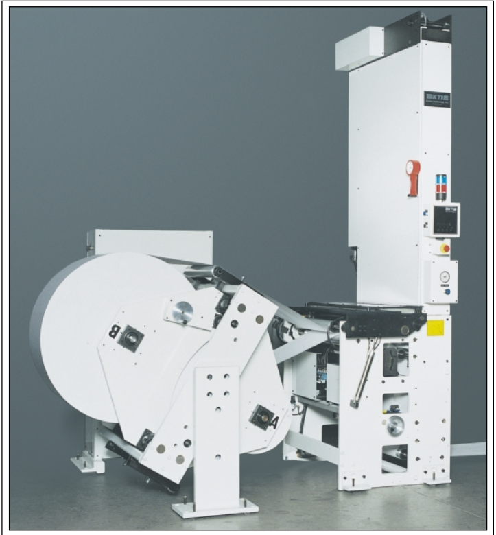
Shown: ZG 2040-05, Butt Splicer for Tag and Label
